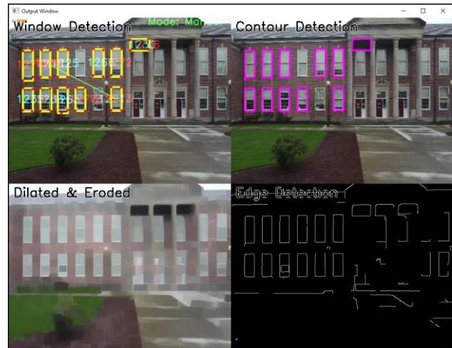
Figure 4.5 – The output window when the CV programme is fed a real video [2] from a drone.
