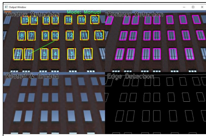
Figure 4.2 – The output window showing the real time images at various stages in the computer vision process. The top right output shows the initial image overlaid with the final window tracking and force vectoring line.
